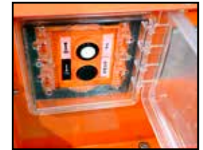
Raise/Lower Switch located on the side of the battery box.
