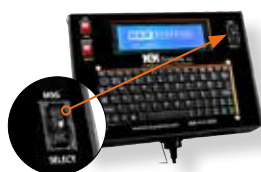
Quick Selection Thumb Wheel for Vehicle Models
