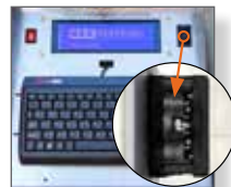
Quick Selection Thumb Wheel for Trailer Mount Keyboard Models
